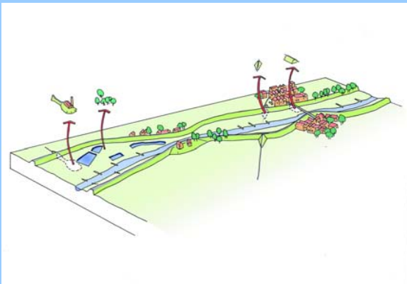
Lowering of floodplains
